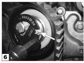
Using an allen key, turn the belt tensioner **anti-clockwise** to a position where the 'window' is aligned with the 'groove'. Tighten the tensioner pulley bolt.
