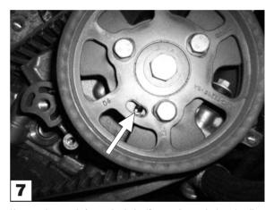
Unscrew the camshaft sprocket bolts (3 on each sprocket) to visually check that they are not at the end of the slotted holes.
