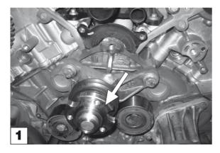
**NOTE**: PSA applications use AST4965C9 Coolant Pump Locking Pin when removing the Pulley. Align one of the three holes in the pulley with the hole in the coolant pump body — insert AST4965C9 Locking Pin to fix position, and remove the pulley.
