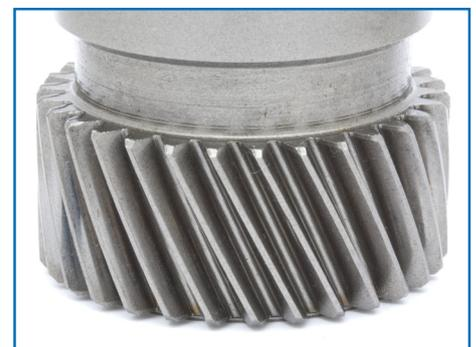
Sun Gear from Toyota Prius showing no wear after 100,000 mile field test.
