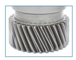
Sun Gear from Toyota Prius showing no wear after 100,000 mile field test.
